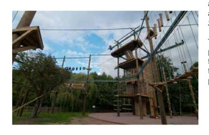
The high ropes adventure course will be a series of obstacles supported on wires that in turn are suspended between timber posts. As the cable system does not need a large steel structure to support itself the course will have very little visual impact particularly as it will be sandwiched between the existing and newly planted trees to the south and trees and range netting to the north.
